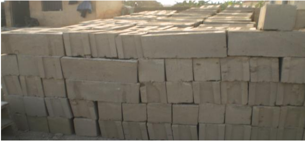
Figure 8: Stacked cured blocks ready for transportation to site.
