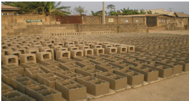
Figure 6: Blocks at curing section.
